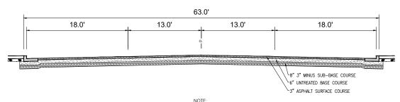
${\sf NOTE:}$  ALL DEPTH STANDARDS ARE MINIMUM AND MORE CAN BE REQUIRED BASED ON GEOTECHNICAL REPORT
