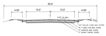
${\tt NOTE:}$  ALL DEPTH STANDARDS ARE MINIMUM AND MORE CAN BE REQUIRED BASED ON GEOTECHNICAL REPORT
